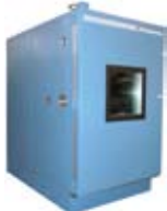
Solar Panel and Photovoltaic Module Test Chambers
